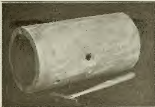
Fig. 26. Five inch tile with small opening, and hammer used in making the opening.
